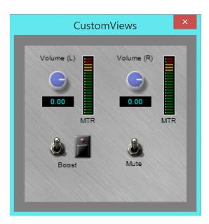
You can see that all the controls are embedded in a CViewContainer object with a lightgreymetal background. There are 2 RackAFX Knob Groups, 2 LED meters, 2 Boost buttons and 1 Mute button.
